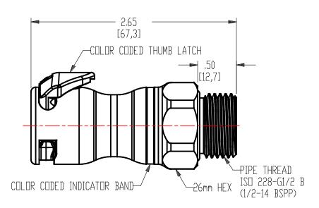
Description: 1/2" G-Thread/BSPP Valved In-line Liquid Cooling Body, Warm Red
