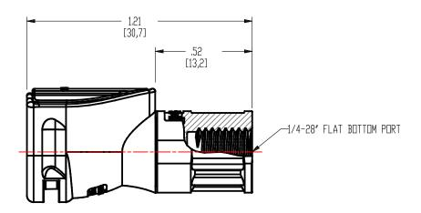
**Description:** 1/4-28" Flat Bottom Port Valved In-Line Coupling Body
