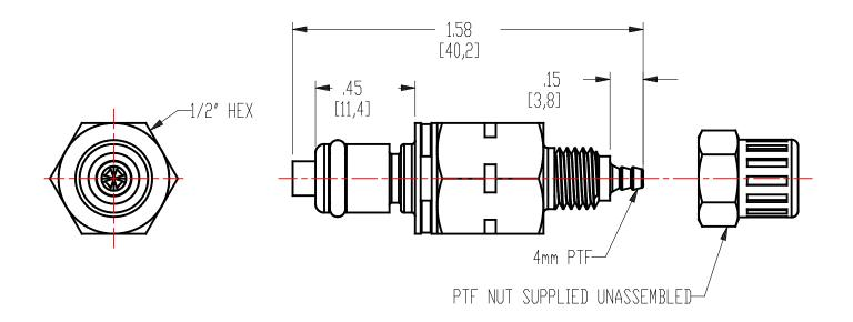
**Description:** 4mm PTF Valved In-Line Coupling Insert
