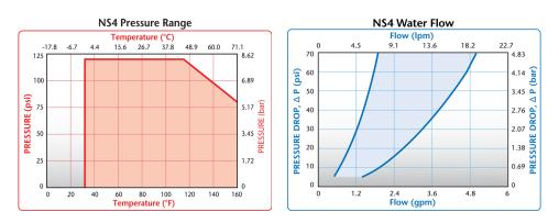
These graphs are intended to give you a general idea of the performance capabilities of each product line. Contact CPC for flow of a particular coupling combination.
